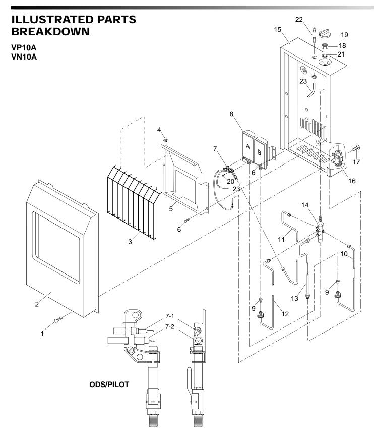
This list contains replaceable parts used in your heater. When ordering parts, follow the instructions listed under *Replacement Parts* on page 28 of this manual.
